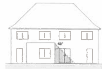
Not acceptable because the centre of the window is within the 45° lines
